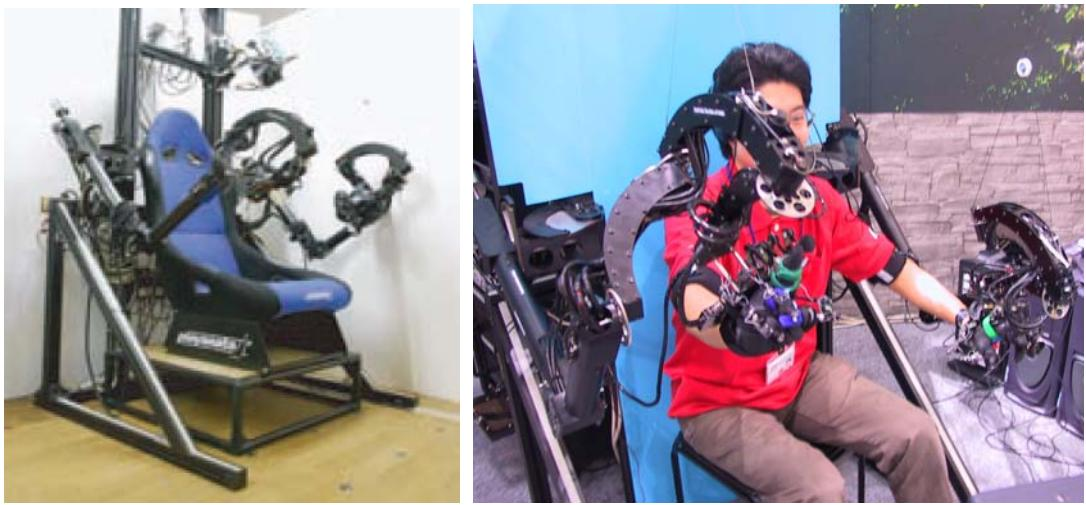
Fig.5 Master arm for TELESAR II : master-slave system (Expo 2005)
