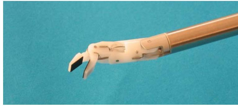
Fig.15 4 D.O.F.  $\phi$ 10 Robotic Forceps Tip (2007)
