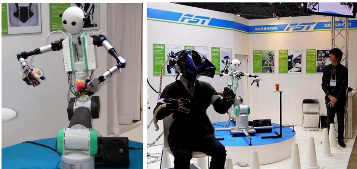
Fig.6 Humanoid robot for TELESAR V : master-slave system (Int. Robot Ex. 2011)
